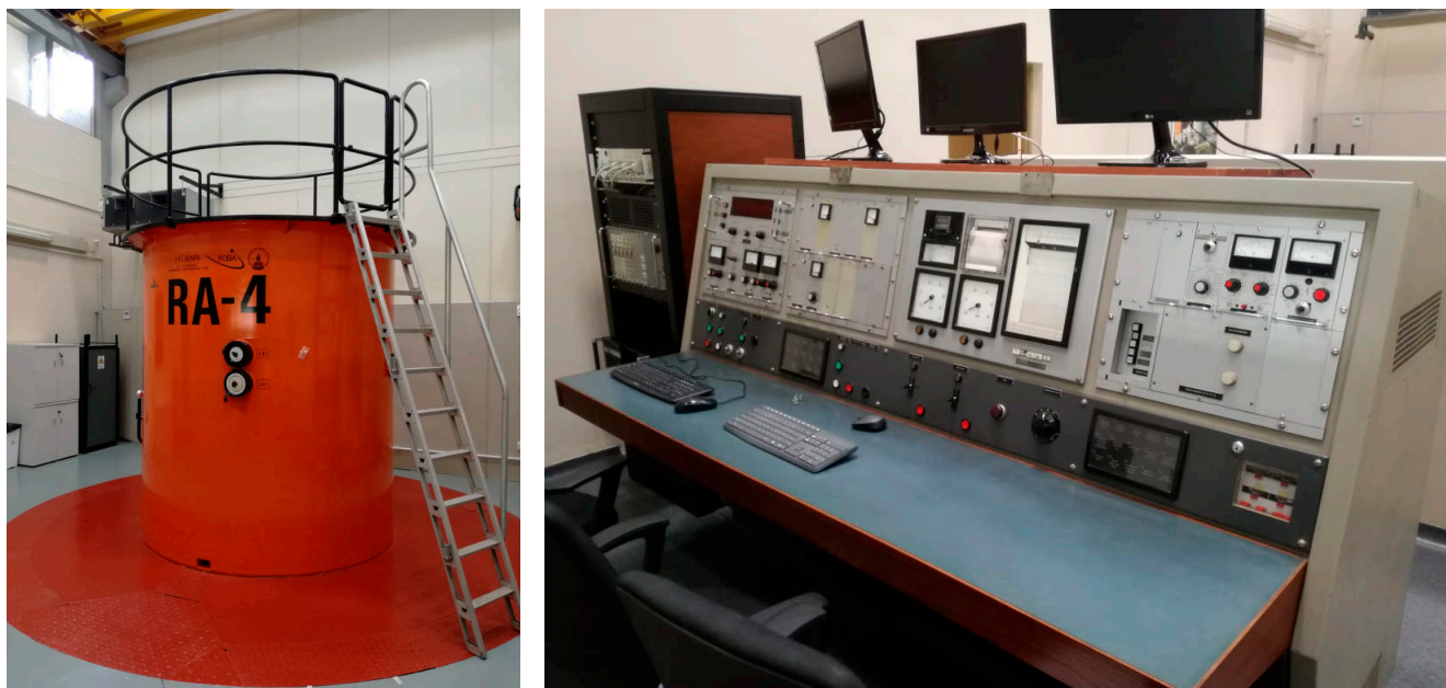
Figure 4: The teaching reactor RA-4 at the Instituto de Estudios Nucleares y Radiaciones Ionizantes IENRI. Credits: Ing. Oscar Peire.
